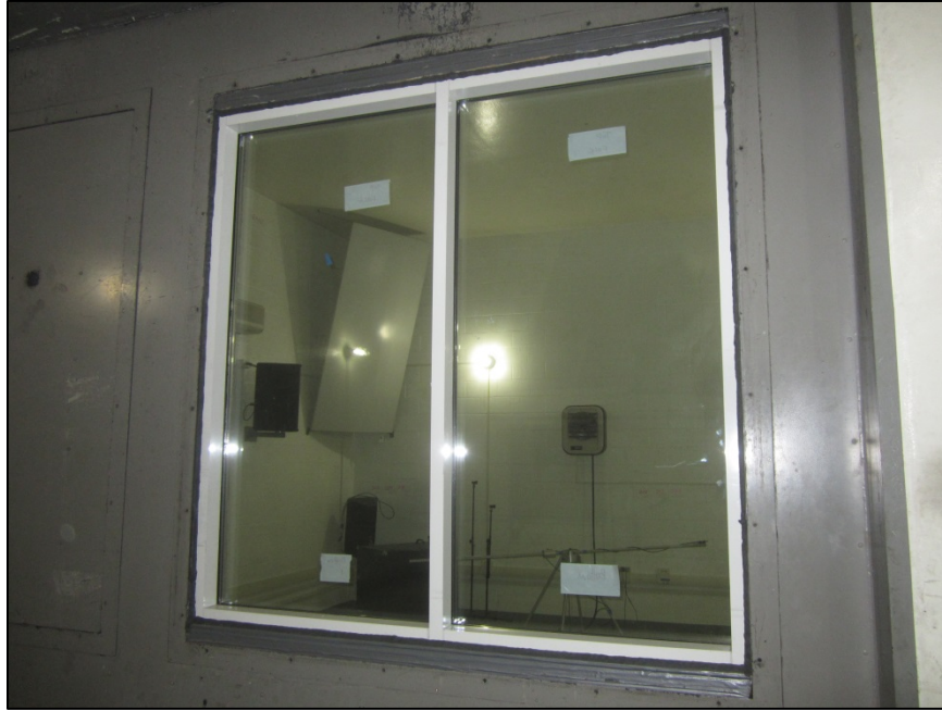
Receive Room View of Installed Test Specimen
